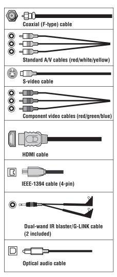
**Note:** Although your TV includes both HDMI and IEEE-1394 connections, it may not operate with another device you have that includes such a connection. For example, the IEEE-1394 ports are not intended to operate with current model Mini DV camcorders, and the HDMI input is not intended for connection to a computer. Copyright protection requirements may also prohibit or limit connectivity. See page 19 for details about the HDMI input. See pages 22–24 for details about the IEEE-1394 ports.
