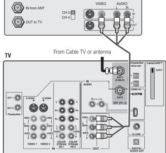
Note: The VIDEO/AUDIO OUT jacks output the signals from the ANT 1, ANT 2, VIDEO 1, VIDEO 2, or VIDEO 3 jacks when the appropriate input mode is selected.
