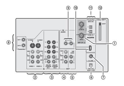
ANT-1 (CABLE) IN and ANT-2 IN — Two inputs that support analog (NTSC) and digital (ATSC) off-air antenna signals and analog and digital (QAM) Cable TV signals.
