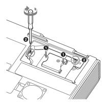
**5** Close the lamp cover and tighten the 1 screw.
