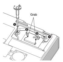
4 Insert the new lamp all the way in until it is securely in place (1). Tighten the 2 screws (2).
