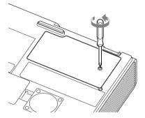
**3** Loosen the 2 screws on the lamp (**1**) then pull out the lamp by its grab (**2**).
