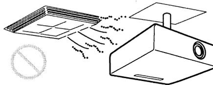
Installing the projector in such a location may cause a malfunction of the unit due to moisture condensation or rise in temperature.
