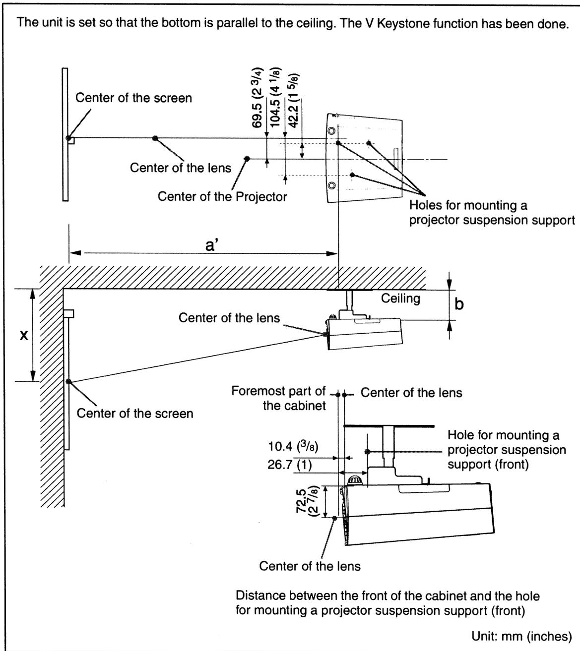
This section describes the examples for installing the projector on the ceiling. When installing the projector on the ceiling, use a Projector Suspension Support recommended by Sony.
