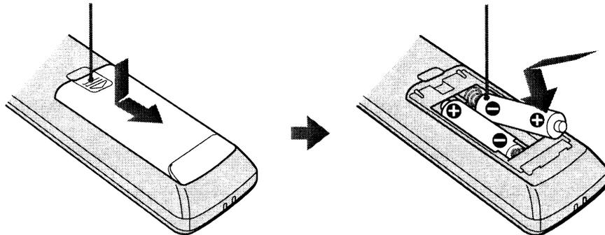
Insert the batteries **+** side first as shown in the illustration. Inserting them forcibly or with the polarities reversed may cause a short circuit and may generate heat.
