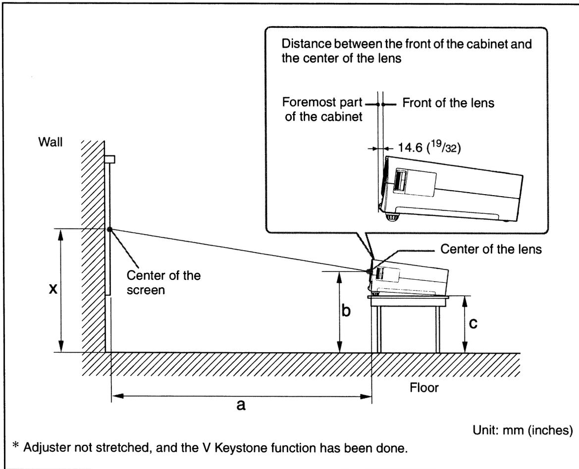
This section describes the examples of installing the projector on a desk, etc.
