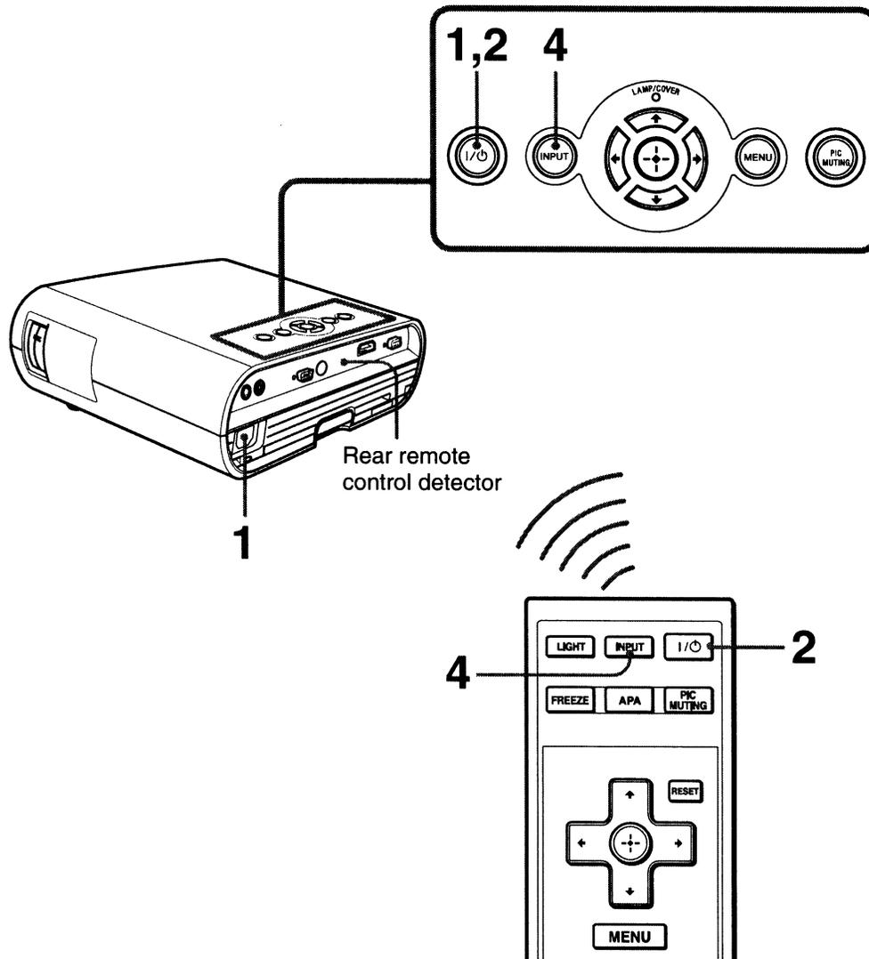
**1** After connecting the AC cord to the projector, plug the AC cord into a wall outlet, connect all equipment, and remove the lens cover.
