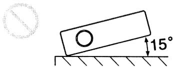
Avoid tilting the unit to an angle of 15°, and avoid installing the unit in any way other than placing it on a level surface or suspending from the ceiling. Such an installation may cause color shading or shorten the lamp life excessively.
