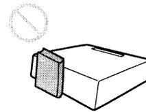
Do not place any object just in front of the lens that may block the light during projection. Heat from the light may damage the object. Use the PIC MUTING button to cut off the picture.
