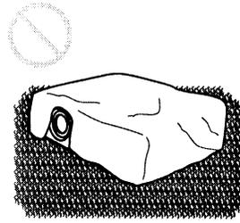
Avoid using a thick-piled carpet or anything that covers the ventilation holes (exhaust/intake); otherwise, internal heat may build up.
