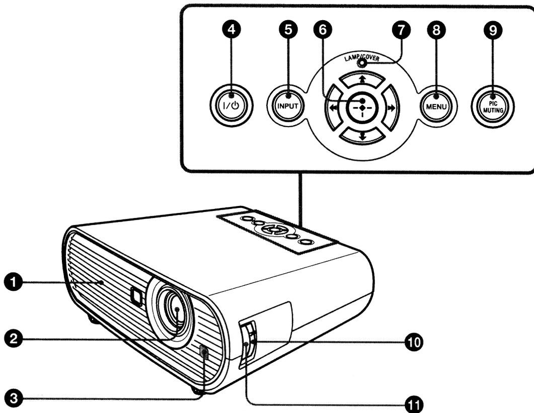
**1 Ventilation holes (exhaust)****2 Lens**
