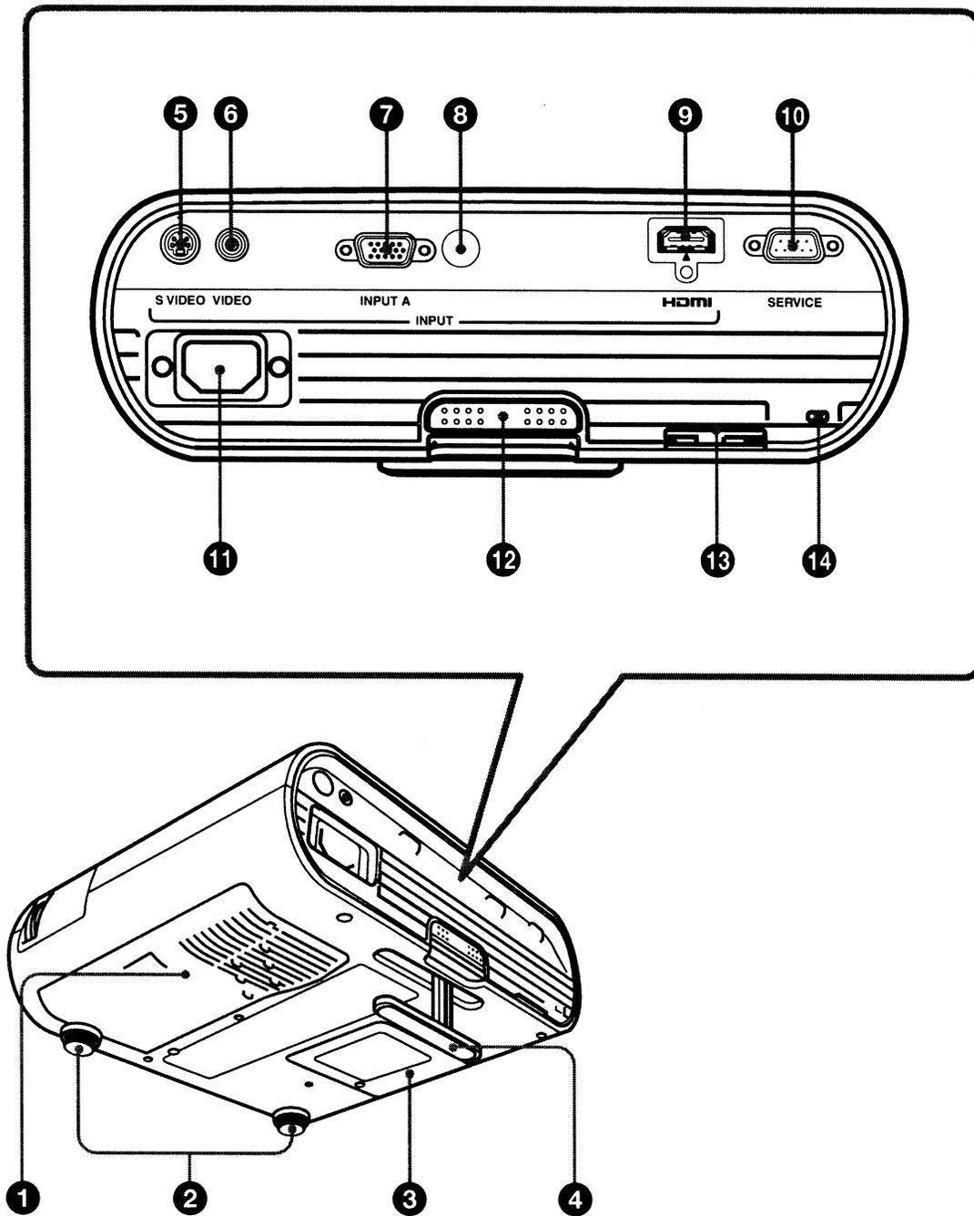
**1 Ventilation holes (intake)/Air filter cover****2 Adjusters (fore pad)****3 Lamp cover****4 Adjuster**
