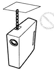
Use the Security bar at the rear of the projector for a purpose of preventing theft, by attaching a commercially available theft prevention cable for example. If you lift the projector by holding the Security bar, or hang the projector by using this bar, it may cause the projector to fall or be damaged.
