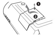
4 Loosen the three screws on the lamp unit with the Philips screwdriver ①. Pull out the lamp unit by the handle ②.
