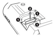
5 Insert the new lamp all the way in until it is securely in place ①. Tighten the three screws ②. Fold down the handle.
