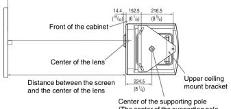
Center of the supporting pole (The center of the supporting pole is different from that of the unit.)
