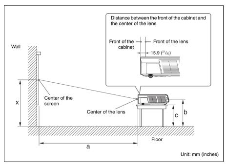
This section describes the examples of installing the projector on a desk, etc.
