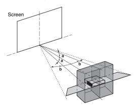
**a:** Tilting angle of the projector in the "V Keystone" adjustment area
