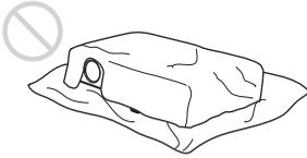
Avoid using something to cover over the ventilation holes (exhaust/intake); otherwise, the internal heat may build up.
