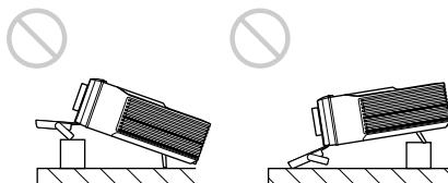
Do not install the unit other than on the floor. Avoid using as the unit tilts upward or downward. These installation may cause malfunction.
