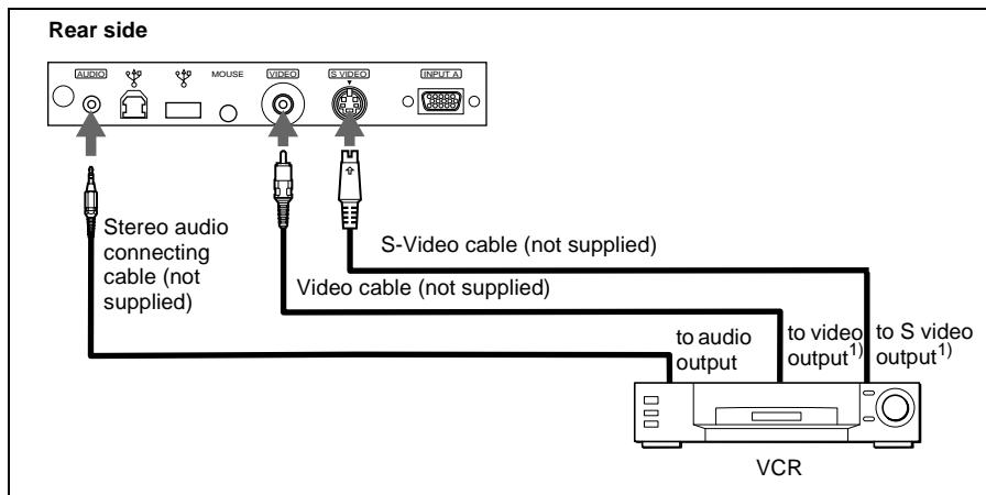
1)When both the S VIDEO and VIDEO jacks are connected to the external equipment, the input signal from the S VIDEO jack is selected.
