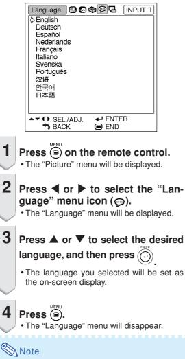
• This procedure can also be performed by using the buttons on the projector.
