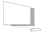
**3** Align the edge of the screen closest to the projector with the test pattern by adjusting the zoom and the adjsuter. (See pages 30 and 31.)
