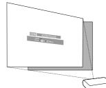
2 Change the projection angle moving the projector or using the adjuster to properly project images onto the screen. (See page 31).
