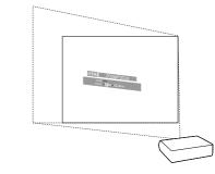
6 Adjust the focus so that the projected image is in focus at the center of the screen. (See page 30.)
