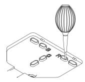
The nozzle will go no further than a certain point when it is put into the hole. Do not attempt to push the nozzle further in, or it could break and be stuck inside of the projector.
