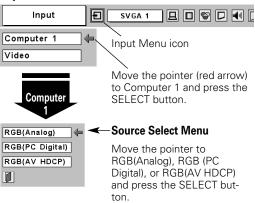
Computer 2 is not displayed when the COMPUTER IN 2/COMPONENT IN/MONITOR OUT terminal is used as Monitor out.
