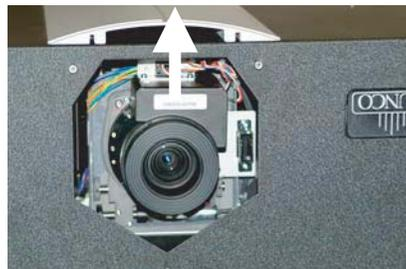
9. Carefully rotate the lens assembly 90 degrees clockwise until the motor socket connector is aligned with the connector on the flange. Then, gently push the lens assembly in until it is seated flush against the flange and the connectors have seated.
