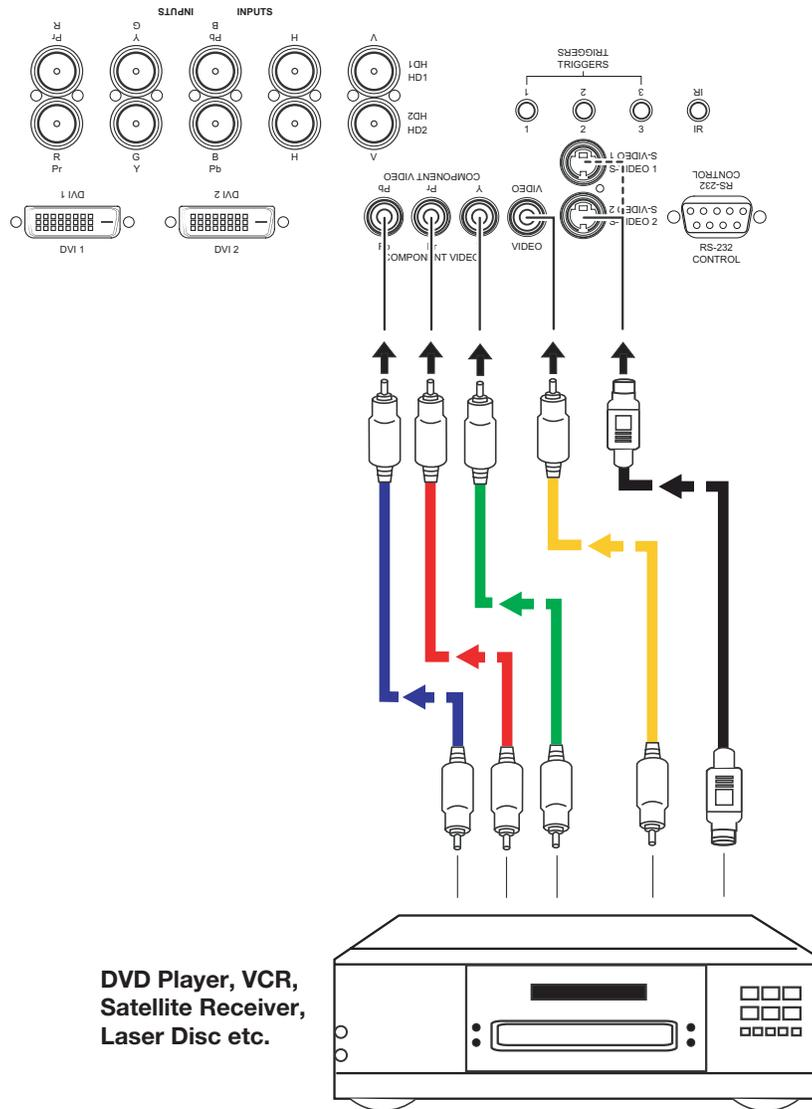
**Figure 3-9. Composite, S-Video and Component Video Connections**
