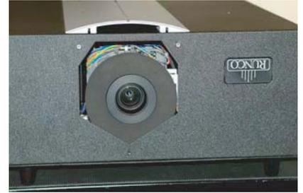
12. Reattach the front lens bezel by sliding the top down onto the two retaining dowels.
