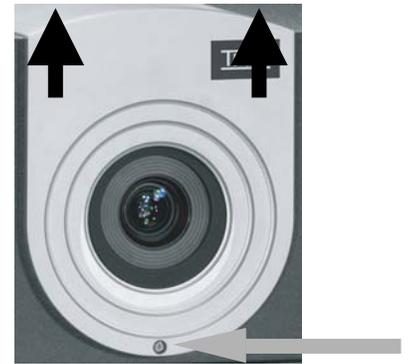
4. Slide the bezel upward to remove it.
