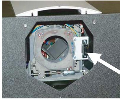
Note that the lens assembly motor has a male socket connector.
