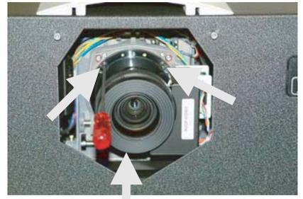
7. Gently pull the lens assembly straight out, just far enough to separate the motor socket connector (on the lens) from the lens mount flange (inside the projector). Then, carefully rotate the lens assembly 90 degrees counter-clockwise (in order to clear the Projector chassis with the Motor Assembly) and remove it.
