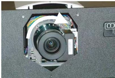
10. Secure the lens assembly to the projector flange with the three Allen screws that you loosened in Step 6.
