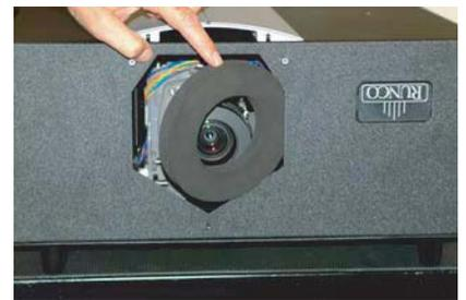
6. Using the red-handled, 3-mm hex driver provided with the projector, loosen the three, captive Allen screws on the outer ring of the lens assembly.
