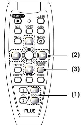
**(2) Pressing the SELECT (▲▼◀▶) buttons on the remote control at the time of the zoom operation will cause the display position to move.**
