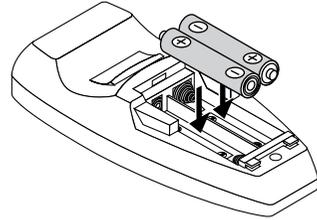
**3** (A) Leaving a little space in the front, close the lid, (B) then with the back pressed tightly, (C) press the lid towards the front.
