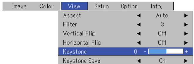
Adjustment display: Each press of the button results in a change of 1 point and continued presses cause changes to proceed in order.
