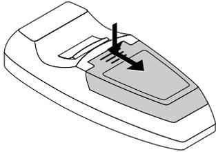
**2** Insert the batteries to match the "+" and "-" as indicated inside the compartment.
