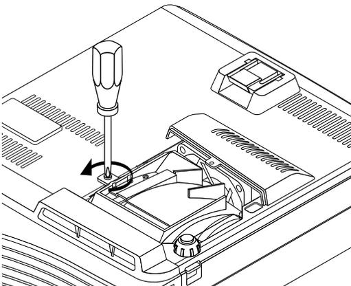
(2) Grasp the lamp cartridge's handle and pull upward to remove the lamp cartridge.
