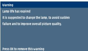
When operation time reaches the last 100 hours of the average lamp life, the message 'Warning: lamp life has almost expired' will be displayed on the screen, each time the projector is switched on. The lamp indicator lights up orange.
