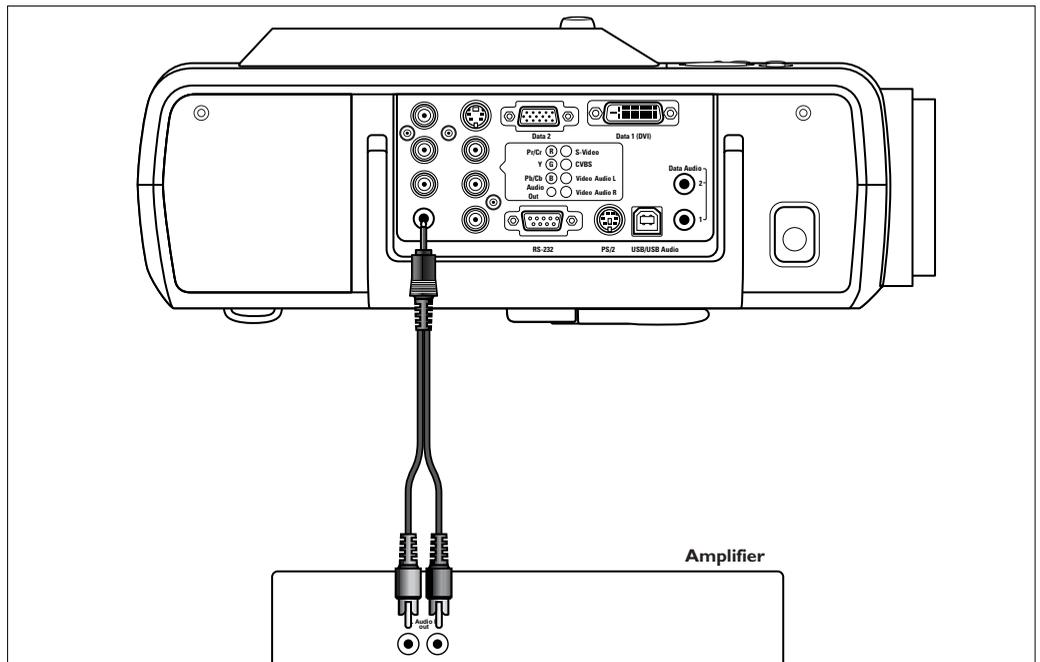
**1** Connect the Audio in L/R sockets of an amplifier or stereo system to the Audio Out socket of the projector.
