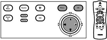
All video and data adjustments and settings (except AV Mute) are done via *On Screen Displays* and with help of Menu, OK and Cursor Control on the projector or the remote control. The projector is set to standard settings at the factory. However, you can adjust these settings to suit your own preferences.
