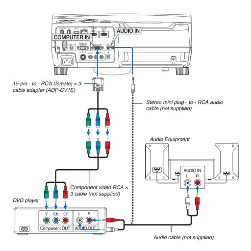
A component signal will be automatically displayed. If not, from the menu, select [SETUP]  $\rightarrow$  [OPTIONS(1)]  $\rightarrow$  [SIGNAL SELECT]  $\rightarrow$  [COMPUTER], and then place a check mark in the Component radio button.
