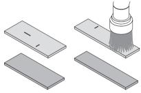
4. Remove dust from the filter cover and the two filter cases (large and small).
