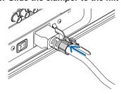
Removing the power cord from the power cord stopper
