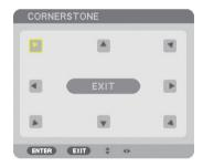
This option allows you to correct trapezoidal distortion. Selecting this item will display the Cornerstone adjustment screen. ( $\rightarrow$  page 37)
