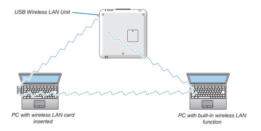
To enable direct communication (i.e., peer-to-peer) between computers and projectors, you need to select the Ad Hoc mode. ( $\rightarrow$  page 136)
