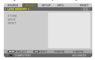
This function serves to store the adjusted values for each input signal when using the LENS SHIFT, ZOOM and FO-CUS buttons of the projector or the remote control. Adjusted values can be applied to the signal you selected. This will eliminate the need to adjust lens shift, focus, and zoom at the time of source selection.
