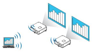
"Easy Connection" function for connecting wireless LAN
