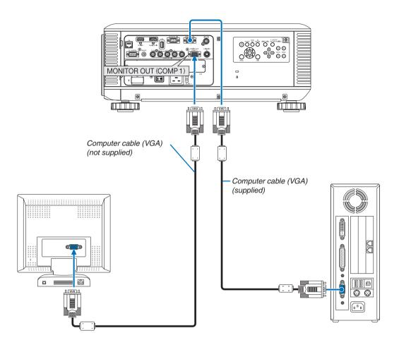
You can connect a separate, external monitor to your projector to simultaneously view on a monitor the computer analog image you're projecting.
