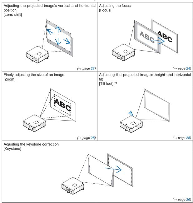
NOTE\*1: Adjust the projected image's height using the tilt feet when you want to project the image at a position higher than the lens shift adjustment range.
