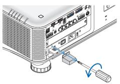
3. Pull out the Wireless LAN Unit from the USB (LAN) port.
