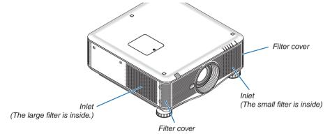
1. Push the positions shown (2 locations) to release the filter cover and remove it.
