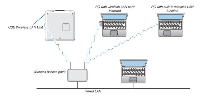
Example of wireless LAN connection (Network Type → Ad Hoc)
