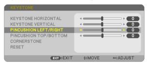
3. Press the ◀ or ▶ button to correct distortion.
