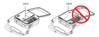
NOTE: When placing the projector in the soft case, retract the tilt foot and the rear feet. Failure to do so may case damage to the projector.
