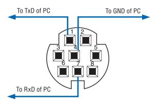
NOTE: Pins 2, 3, 5, 6 and 8 are used inside the projector.
