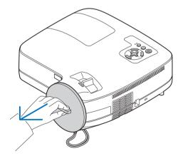
2. To turn on the main power to the projector, press the Main Power switch to the on position (1).
