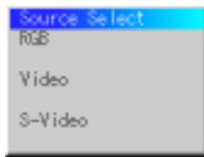
Enables you to select a video source such as a VCR, DVD player, laser disc player, computer or document camera depending on what is connected to your inputs. Press the “Select” button on the projector cabinet or ▲▼ buttons on your remote control to highlight the menu for the item you want to adjust.
