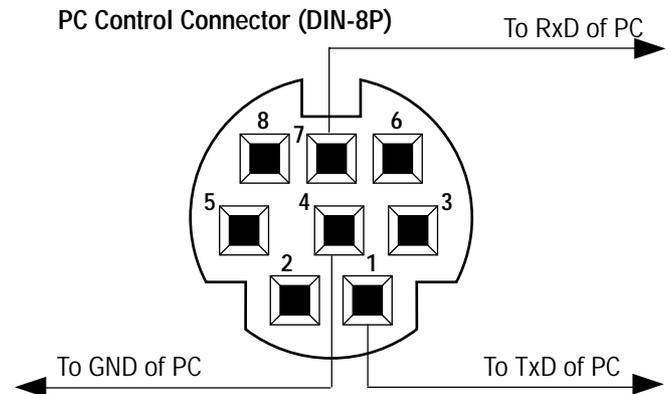
**NOTE:** Pins 2, 3, 5, 6 and 8 are used inside the projector.
