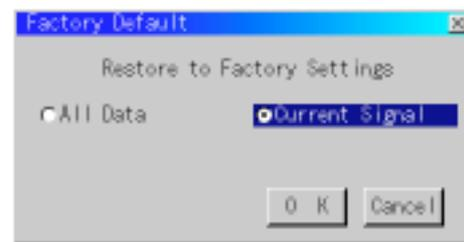
Changes all adjustments and setting to the factory preset for each source individually except Lamp Usage Hours. (To reset the lamp usage time, see “Clear Lamp Hour Meter” on page E-32.)
