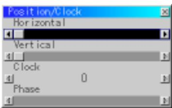
This allows you to manually adjust the image horizontally and vertically, and adjust Clock and Phase.
