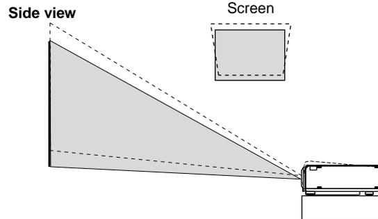
(There is approximately 10 degrees of up and down adjustment for the front of the projector.)
