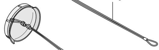
3. Use the rivet to attach the string to the bottom of the lens hood.
