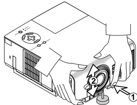
To fine-tune the image's position vertically on the screen, rotate the foot. Each of the rear feet height can be changed up to 0.6" (4mm).
