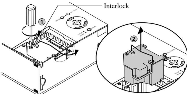
3. Insert a new lamp housing until the lamp housing is plugged into the socket.
