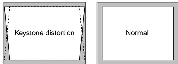
**NOTE:** The maximum keystone angle that can be corrected is 15 degrees upward and downward with the projector placed horizontally. However, a picture will be blurred if you correct the keystone angle beyond +12 degrees or more for SXGA signal on VT440.
