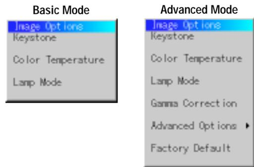
Provides optional controls such as Keystone Correction, Color Temperature and Lamp Mode. When you select Advanced Mode, the following options are available: Gamma Correction, Aspect Ratio, Noise Reduction, Color Matrix, White Balance, Auto Adjust, Position/Clock, Resolution, and Factory Default.
