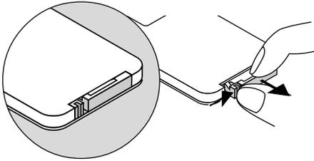
2. Remove the old Lithium coin cell and install new one (CR2025). Ensure that the side with a “+” is facing up.
