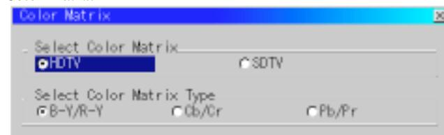
First select an appropriate color matrix to fit your component signal for HDTV or SDTV. Then select an appropriate matrix type from B-Y/R-Y, Cb/Cr or Pb/Pr.
