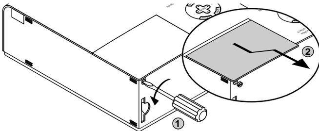
2. Loosen the two screws securing the lamp housing until the screwdriver goes into a freewheeling condition. The two screws are not removable.
