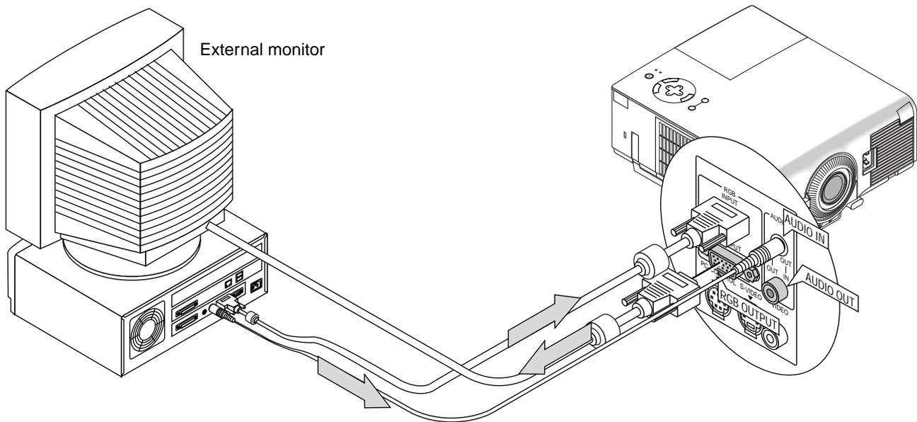
You can connect a separate, external monitor to your VT440/VT540 to simultaneously view on a monitor the image you're projecting. To do so:
