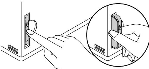
**NOTE:** Do not push or pull the card remote control in a slanting direction. Unless you push the card remote control straight, you may not eject the card remote control. Should this happen, try pushing the card remote control straight again.
