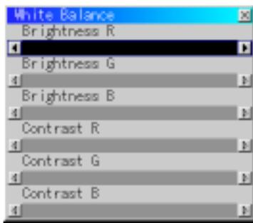
This allows you to adjust the white balance. Brightness for each color (RGB) is used to adjust the black level of the screen; Contrast for each color (RGB) to adjust the white level of the screen.
