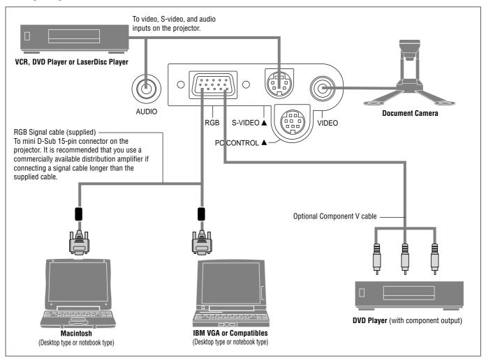
NOTE: When using with a notebook PC, be sure to connect between the projector and the notebook PC before turning on the power to the notebook PC. In most cases signal cannot be output from RGB output unless the notebook PC is turned on after connecting with the projector.
