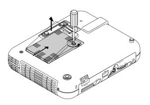
2 Loosen the three screws securing the lamp housing until the screwdriver goes into a freewheeling condition. The three screws are not removable.
