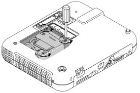
3 Remove the lamp housing by pulling out the handle. *NOTE:* There is an interlock on this case to prevent the risk of electrical shock. Do not attempt to circumvent this interlock.
