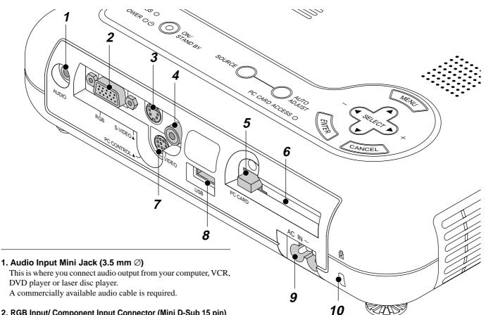
**2. RGB Input/ Component Input Connector (Mini D-Sub 15 pin)** Connect your PC or other RGB equipment such as IBM or compatible computers. Use the supplied RGB cable to connect to a PC. Or connect a Macintosh computer here using the supplied RGB cable. This also serves as a component input connector that allows you to connect a component video output of component equipment such as a DVD player.
