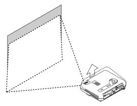
*Lift the front edge of the projector to center the image vertically.*
