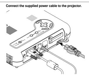
Plug the supplied power cable in the wall outlet. The projector will go into its standby mode and the power indicator will glow orange.
