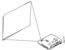
Rotate the rear foot to make the image square to the screen.
