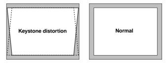
NOTE: The maximum keystone angle that can be corrected is 45 degrees upward and 15 degrees downward with the projector placed horizontally on the ground plane.
