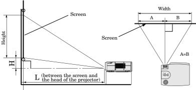
To find the approximate distance between the projector and screen: Multiply the width of the screen x 1.8 (min.) , Multiply the width of the screen x 2.2 (max.).
