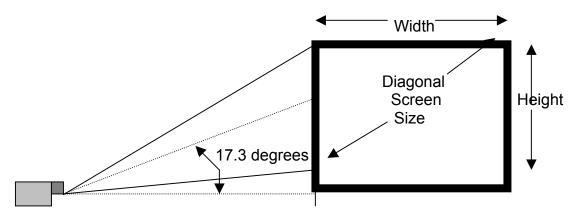
Use the following information to position the projector. Horizontally the projector needs to be positions with the lens-centered left to right
