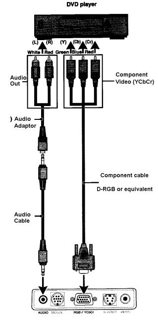
You can also connect the video component to the RGB IN connector, if the video component has the component video (YCbCr) signal jacks. This connection may provide a better picture quality than the connections on page 8.
