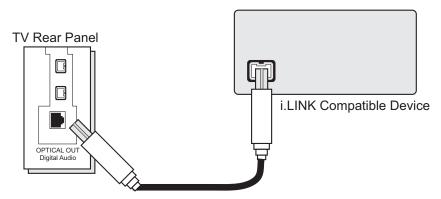
Connect the i.LINK cable from the back of the TV to the back of the i.LINK compatible device
