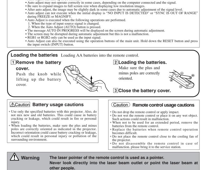
The laser beam can cause vision problems.
