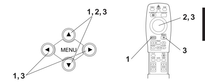
**1** Press the MENU ( ( ) ) buttons of the projector or the MENU button of the remote control.
