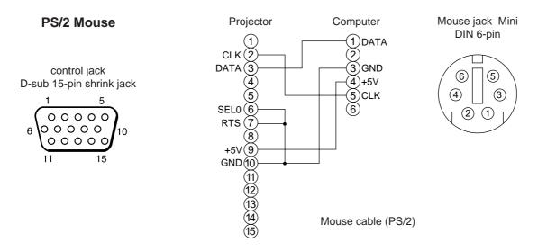
Use the mouse cable provided or a PS/2 mouse cable (for IBM and compatibles). Cables for ADB mouse (Apple), bus mouse (NEC) and serial mouse are available as options.
