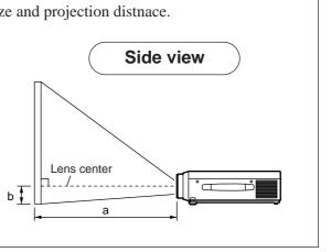
a. Distance from the LCD projector to the screen b. Distance from the lens center to the bottom of the screen (a,b: +/-10%).
