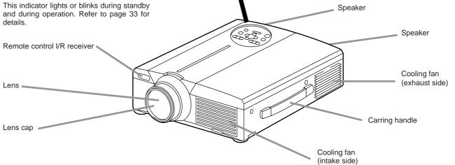
• Use the remote control in front of the remote control photoreceptor at a distance of about 5 m or less and an angle of 30 degrees to the left or right of the center.
