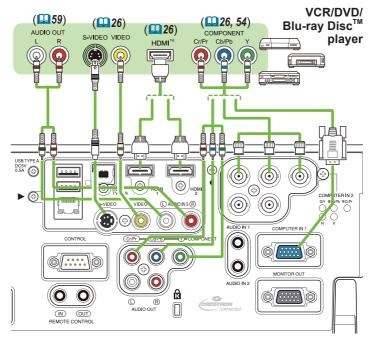
**NOTE** • The **HDMI** ports of this model are compatible with HDCP (High-bandwidth Digital Content Protection) and therefore capable of displaying video signals from HDCP compatible DVD players or the like.
