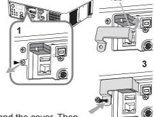
3. Align the screw holes on the projector and the cover. Then insert the screw removed from the projector into the hole and tighten the screw.
