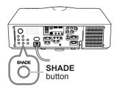
**△CAUTION** ► If you wish to have a blank screen while the projector's lamp is on, use the lens shade function above or the AV MUTE function (☐25). Taking any other action may cause the damage on the projector.
