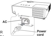
**△WARNING** ► Please use extra caution when connecting the power cord, as incorrect or faulty connections may result in fire and/or electrical shock.
