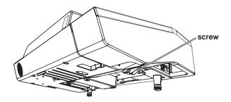
**△CAUTION** ► Be careful not to pinch the cables in the cable cover, to prevent damage to the cables.
