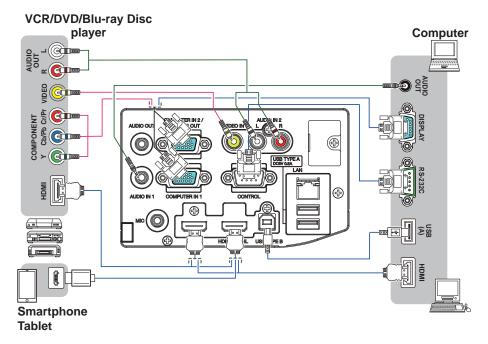
**NOTE** • Before connecting the projector to a computer, consult the computer's manual and check the compatibility of the signal level, the synchronization methods and the display resolution output to the projector.
