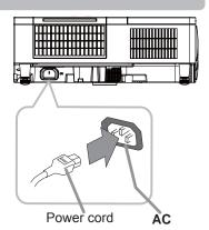
**⚠WARNING** ► Please use extra caution when connecting the power cord, as incorrect or faulty connections may result in fire and/or electrical shock.
