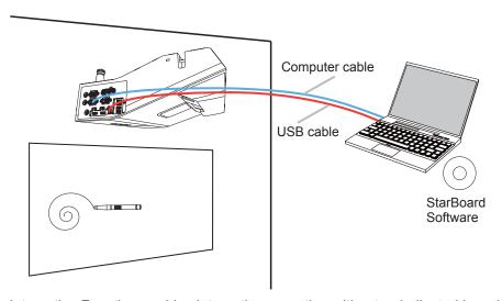
The Interactive Function enables interactive operation without a dedicated board such as the operation on the connected computer or writing on the display with the sensor equipped in the projector and bundled Interactive pen.
