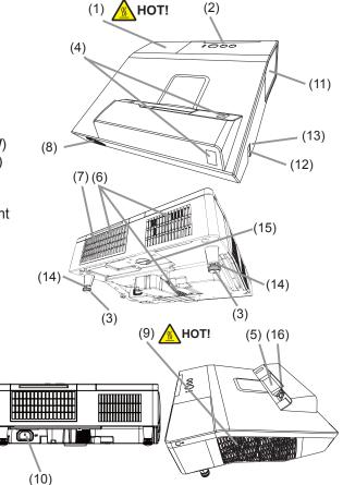
**△WARNING** ► **HOT!** : Do not touch around the lamp cover and the exhaust vents during use or just after use, since it is too hot.
