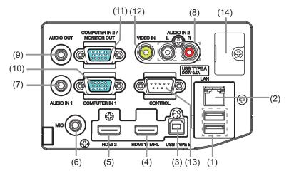
**NOTE** \* Option port is a port used only when using the optional part (FT-01B). A cover is attached for protecting the port. Do not remove the cover. Refer to the manual of the optional part (FT-01B) for detail.
