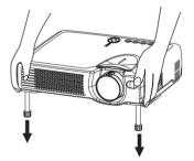
As necessary, you can also finely adjust the height of the projector by twisting the elevator feet by hand
