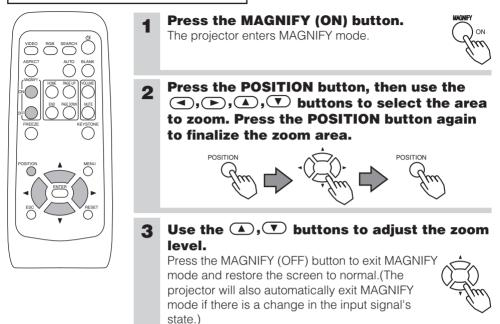
**NOTE** • The projector will automatically exit from MAGNIFY mode if either the SEARCH, RGB, AUTO, ASPECT or VIDEO feature is used, or, if there is a change in the input signal's state.
