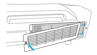
If a message is frequently displayed, even after cleaning, it is time to replace the air filter. Replace it with a new air filter. • p.127
