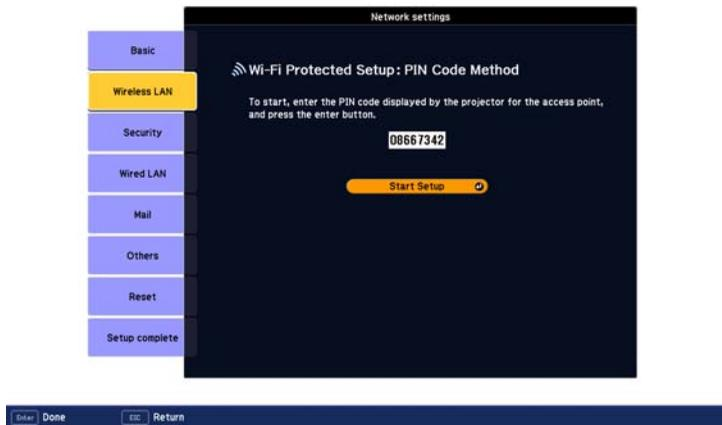
3. From the computer, enter the displayed PIN code for the access point, select **Start Setup** and then press **Enter**.
