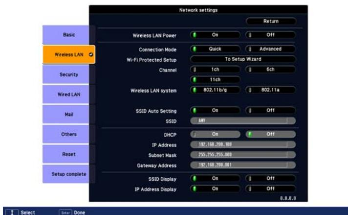
4. Make sure **Wireless LAN Power** is set to **On**. You can turn it off to prevent unauthorized access.
