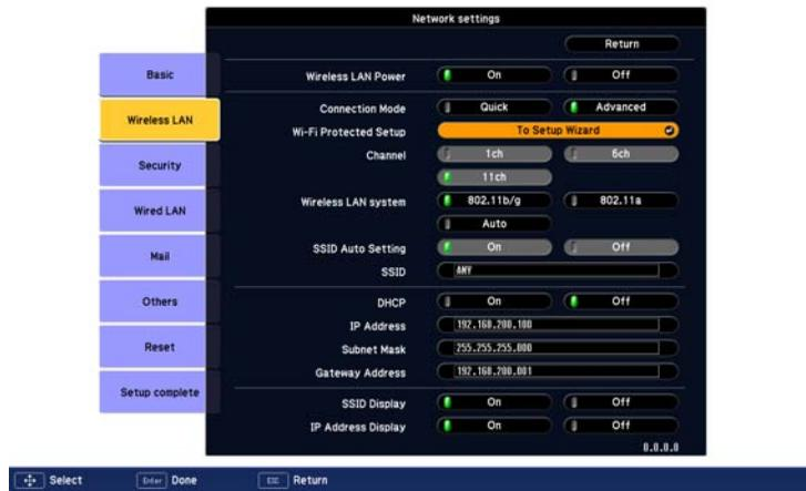
4. Select To Setup Wizard, then press Enter. You see the WPS (Wi-Fi Protected Setup) connection screen:
