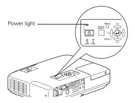
3. Press the red  $\circlearrowleft$  **Power** button on the remote control or on top of the projector.
