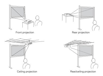
To project from overhead, you'll need the optional ceiling mounting hardware; see page 12 for ordering information. You'll also need to select Front/Ceiling or Rear/Ceiling as the Projection option in the projector's Extended menu to flip the image upside-down. To project from the rear, onto a semi-transparent screen, select Rear or Rear/Ceiling (see page 63).
