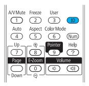
2. While holding the ID button, press the numbered button on the remote control (1 through 9) that corresponds to the ID of the projector(s) you want to operate. Selecting zero lets you control all projectors.
