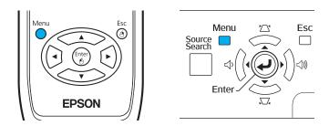
From the Setting menu, select **Keystone** and press **Enter**. Use the pointer button on the remote control to adjust the keystone setting as needed.
