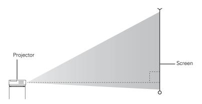
If you place the projector below screen level, you'll have to tilt it up by extending the front adjustable foot. This causes the image to become "keystone" shaped, but you can correct the distortion by pressing the buttons on the projector. See page 23 for detailed information about correcting the image shape.
