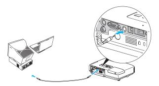
■ For video equipment, use an RCA-style audio cable and the audio adapter included with the projector.
