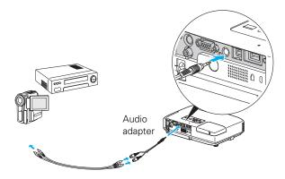
2. Connect the other end of the cable to the audio output connector(s) on your computer or video equipment.
