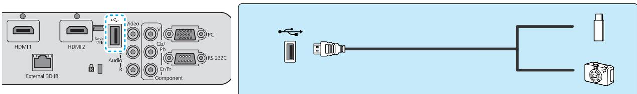
When the USB device is connected, you can project image files on the USB memory or digital camera as a slideshow. [p.51](#)
