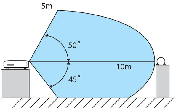
Vertical direction (suspended from a ceiling)
