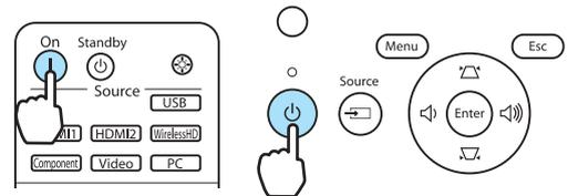
When **Direct Power On** is set to **On**, you can start projecting by simply connecting the power cable to the projector without having to press any buttons. **Extended - Operation - Direct Power On** p.63
