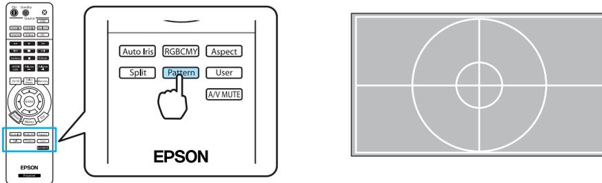
Press the **Esc** button to close the test pattern, or select **Exit**.
