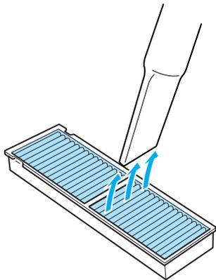
**6** Install the air filter into the air filter cover.
