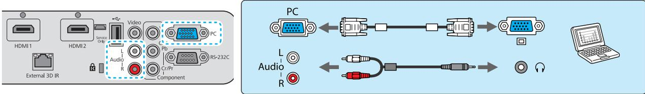
For audio connections, make sure you use an audio cable labeled "No resistance" to connect the 2RCA ↔ stereo mini-plug.
