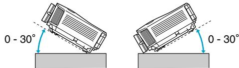
Using the projector at angles not shown in the illustrations above may damage it or cause an accident.
