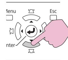
If the [↖/↗] and [↘/↙] buttons are pressed simultaneously for at least 1 second, the value of vertical keystone will return to the original status.
