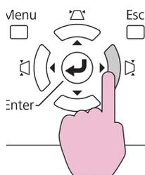
If the [←/→] and [↶/↷] buttons are pressed simultaneously for at least 1 second, the value of horizontal keystone will return to the original status.
