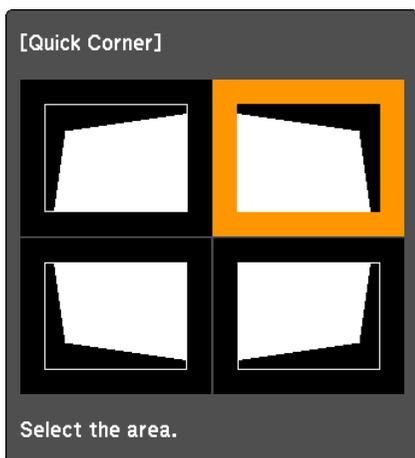
**4** Correct the position of the corner using the [⊙] button on the remote control, or the [△/▲], [▽/▼], [◀/▶] and [↵/↳] buttons on the control panel.
