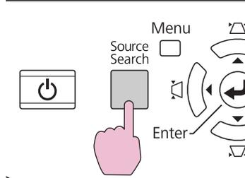
When the [Source Search] button is pressed, a search is made for input ports to which video signals are being input in the following order. (The input port where no image signal is being input is skipped.)
