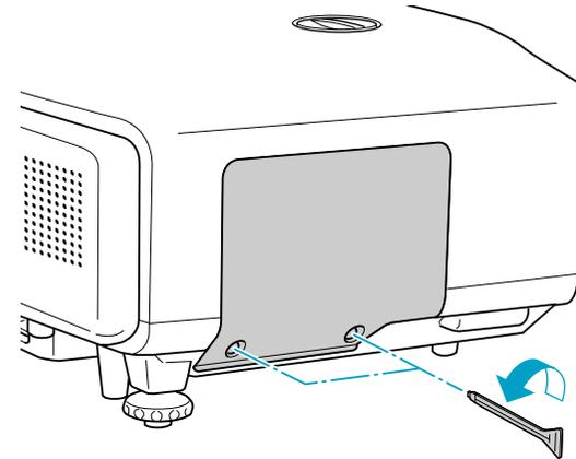
**3** Loosen the two lamp fixing screws.
