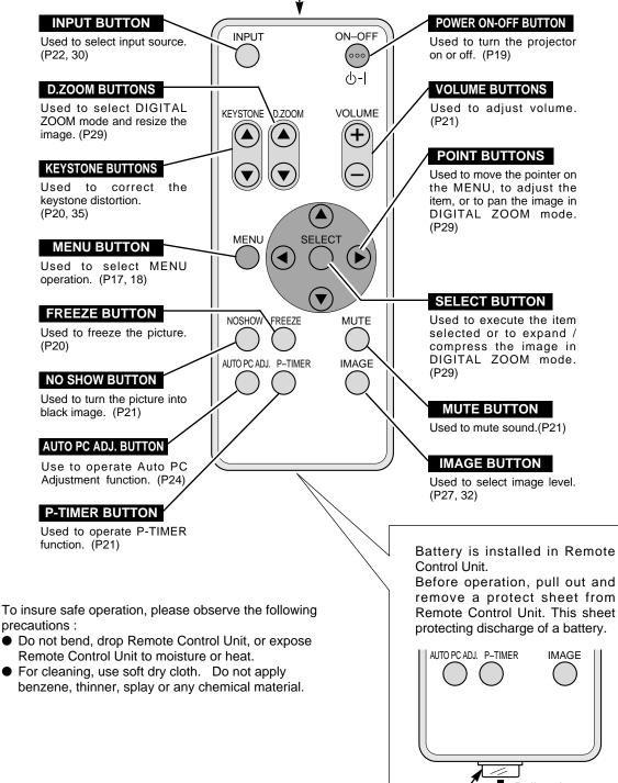
Pull and remove. BATTERY PROTECT SHEET (transparent sheet)
