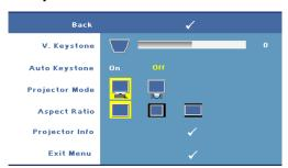
V. KEYSTONE—Allows you to adjust image distortion caused by tilting the projector.
