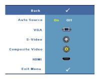
Auto Source—Select On (Default) to automatically detect the available input signals. When **On** is selected and you press Source on the control panel/remote, it automatically finds the next available input signal.
