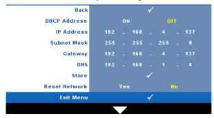
**DHCP ADDRESS**—If a DHCP server exists in the network to which the projector is connected, the IP address will automatically be acquired when you select DHCP On. If DHCP is Off, manually set the IP Address, Subnet Mask, and Gateway. Use to select the number of IP Address, Subnet Mask, and Gateway. Key in Enter to confirm each number and then use  $\bigcirc$  by to set the next item.
