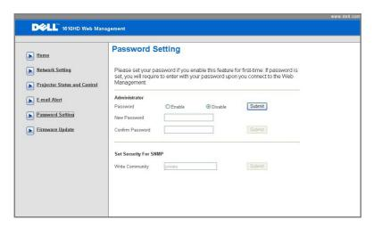
Use Password Setting to set up an administrator password to access the Web Management. When enabling password for the first time, set the password before enabling it. When the password function is enabled, the administrator password will be required for accessing the Web Management.
