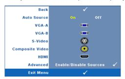
AUTO SOURCE—Select Off (the default) to lock the current input signal. If you press the Source button when the Auto Source mode is set to Off, you can manually select the input signal. Select On to auto detect the available input signals. If you press the Source button when the projector is on, it automatically finds the next available input signal.
