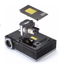
9 Reset the lamp usage time by selecting "Yes" for Lamp Reset in the OSD Lamp tab (see Lamp menu on page 38). When a new lamp module has been changed, the projector will automatically detect and reset the lamp hours.
