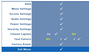
**MENU SETTINGS**—Select and press on the control panel or press **Enter** button on the remote control to activate menu settings. The menu settings consists of the following options:
