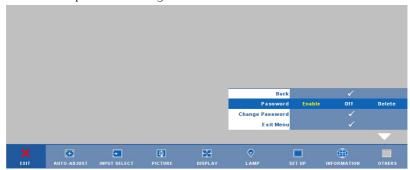
**b** Enabling the Password function will pop up a character screen, key in a 4-digit number from the screen and press on the control panel or press Enter button on the remote control.
