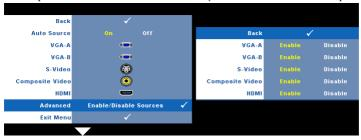
**VGA-A**—Use **<** and **≥** to enable or disable VGA-A input.
