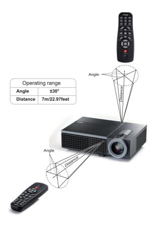
**NOTE:** Actual operating range may slightly differ from the diagram. Weak batteries will also prevent the remote control from properly operating the projector.
