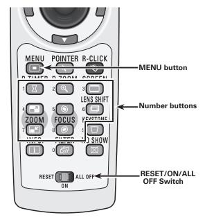
Press and hold the MENU and a number button (1–8) that corresponds to the remote control code for more than five seconds to switch between the codes.
