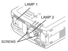
Make sure which number of lamp needs to be replaced on Lamp Status Display. Figure shows case of replacing LAMP 2.
