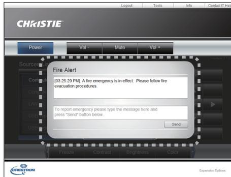
When the administrator for Crestron RoomView® Express sends out an alert message, it will be displayed on the screen. You can reply to the alert message via a chat format. Input a message in the box below the alert message, and click the **[Send]** button.
