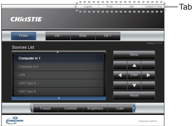
The Main window as shown above is displayed at first. However, if you have enabled User Password on the Tools window (46), a dialog prompting you to enter the password as shown on the right will be displayed, and no operation is enabled until you have entered the password. After entering the preset password, the dialog disappears and the Main window will be displayed. As shown below, you can open a window by clicking the corresponding tab at the top right of the window.
