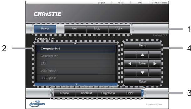
You can operate the basic controls of the projector on this screen.
