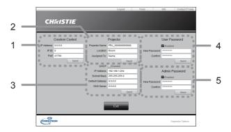
Configures the settings between the projector and Crestron® control system. Click the **[Exit]** button to return to the Main window.
