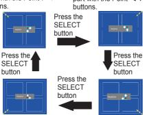
Reduce the bottom left corner part with the Point **b** buttons.
