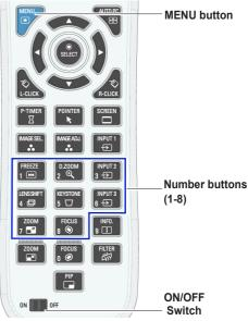
Press and hold the MENU and a number button (1-8) that corresponds to the remote control code for more than five seconds to switch among the codes.
