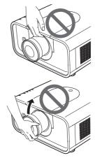
Do not hold the lens and the peripheral part.
