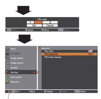
When the projector is locked with a PIN code, the PIN code lock symbol appears in the Guide.
