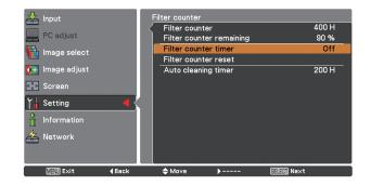
Press the SELECT button to select Filter counter timer and use the Point ▲▼ buttons to set the timer. Select from (Off/ 4000H/ 8000H/ 12000H/16000H) depending on the use environment.
