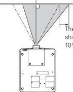
The display position can be shifted to the right in up to 10% width of the display.
