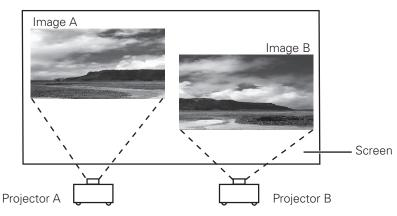
3 If black horizontal and/or vertical bar(s) on four sides of the images appear, adjust the Start values until they become invisible and specify the values for Width to adjust the width of the area where the images overlap. (Refer to pages 58, 59 for operation procedure.)
