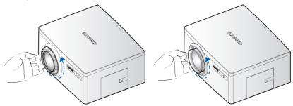
5. **Install the new lens:** Fully insert the lens assembly straight into the lens mount without turning. Rotate the lens cap clockwise to lock the lens in place.
