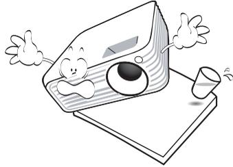
11. Do not attempt to disassemble this projector. There are dangerous high voltages inside which may cause death if you should come into contact with live parts. The only user serviceable part is the lamp which has its own removable cover. Under no circumstances should you ever undo or remove any other covers. Refer servicing only to suitably qualified professional service personnel.
