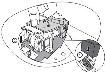
7. Tighten the screw that secures the lamp.
