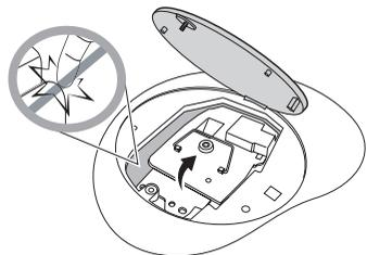
4. Loosen the screw that secures the lamp.
