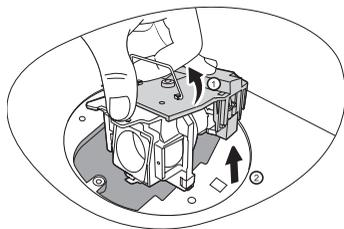
6. As shown in the figure, lower the new lamp first into the connector on the projector and align the two holes on the projector.
