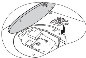
10. Tighten the screw that secures the lamp cover.
