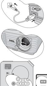
(If necessary) Rotate the focus ring to adjust the image clearness.
