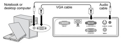
Many notebooks do not turn on their external video ports when connected to a projector. Usually a key combo like FN + F3 or CRT/LCD key turns the external display on/off. Locate a function key labeled CRT/LCD or a function key with a monitor symbol on the notebook. Press FN and the labeled function key simultaneously. Refer to your notebook's documentation to find your notebook's key combination.
