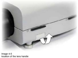
2. Remove the lens out of its housing
