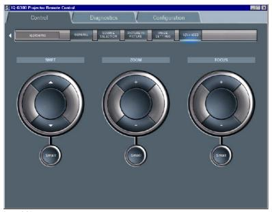
Image 8-21 Use the buttons to choose small, medium or large adjustment steps. Each click changes the setting.
