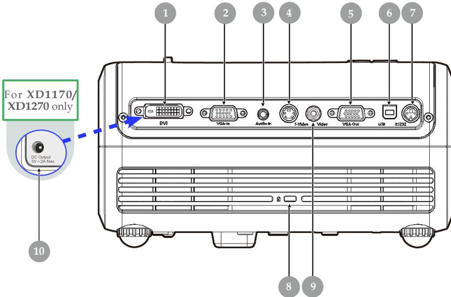
1. DVI Input Connector (for Digital signal with HDCP function) (Optional)
