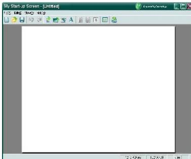
Acer **My Start-up Screen** is a PC utility for user to change the default start-up screen of Acer projector to their desired image. You can install **My Start-up Screen** from the bundled CD. Connect the projector to your PC with the bundled USB cable then execute **My Start-up Screen** utility to download your desired image from your PC to projector. Before the download starts, the projector must enter “Download Mode” first. Please follow the instruction below to enter “Download Mode”.
