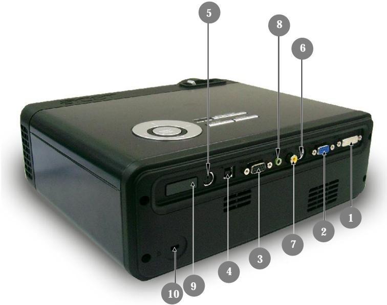
1. DVI-I Input Connector (for Digital signal with HDCP function) (Optional)
