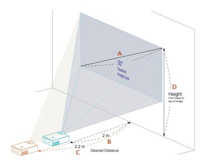
The table below shows how to achieve a desired image size by adjusting either the position or the zoom ring. For example: to obtain an image size of 50" set the projector at a distance 2 m and 2.2 m from the screen and adjust the zoom level accordingly.
